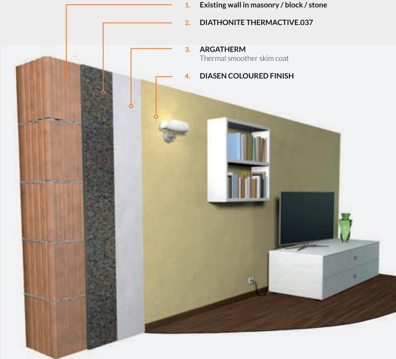
1. Existing wall in masonry / block / stone
