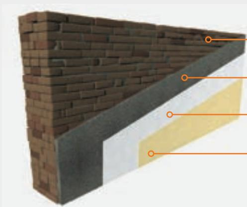
1. Existing wall in masonry /block/ stone
