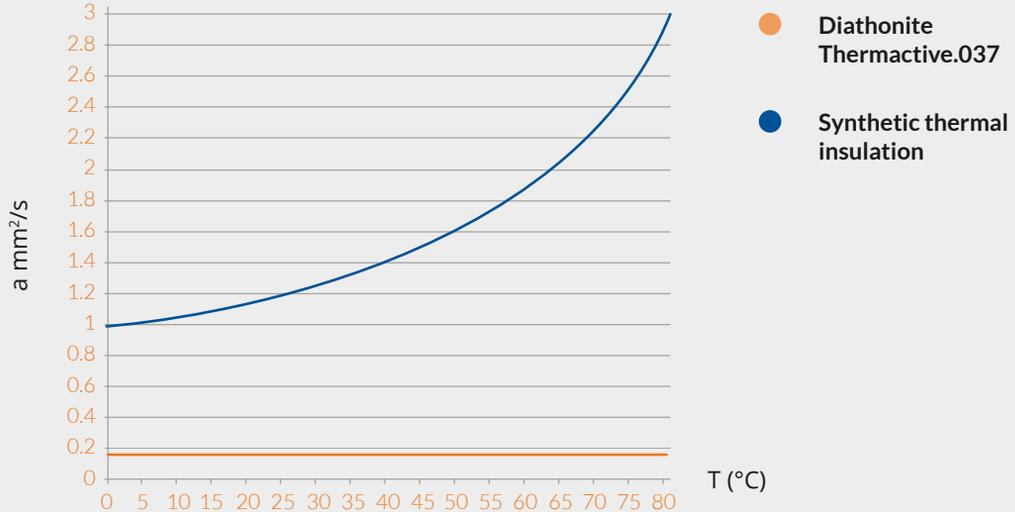
The graphic illustrates how in summer months, when the surface temperature of the exterior insulation even exceeds 60°, the thermal insulating properties of the synthetic materials plummet, allowing transmission of heat to the building interior, with marked deterioration of indoor climate conditions. In this context, the intrinsic characteristics of Diathonite Thermactive.037, meanwhile, provide the insulation from heat which synthetic materials are unable to offer.
