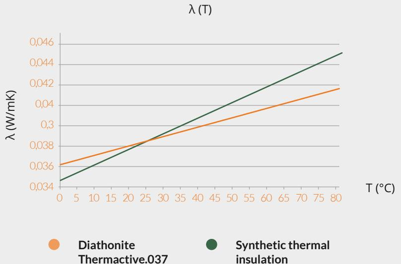
The experimental evaluation of this comparative behaviour was conducted in compliance with the parameters established in **EN ISO 10456:2008**: "Building materials and products - Hygrothermal properties" - Tabulated design values and procedures for determining declared and design thermal values.
