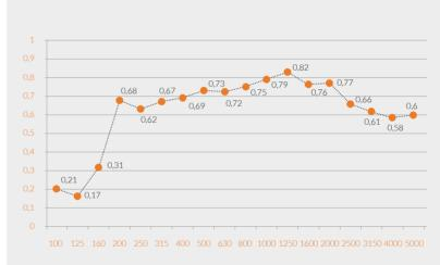
The graph shows a sequence of values that highlight how absorption always exceeds 70% in the speech frequency range (from 500 to 2000 Hz).
